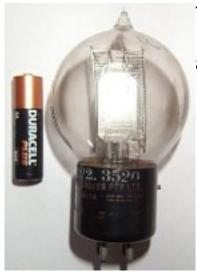
This valve measures 107x55mm overall and has a 4 pin base.
