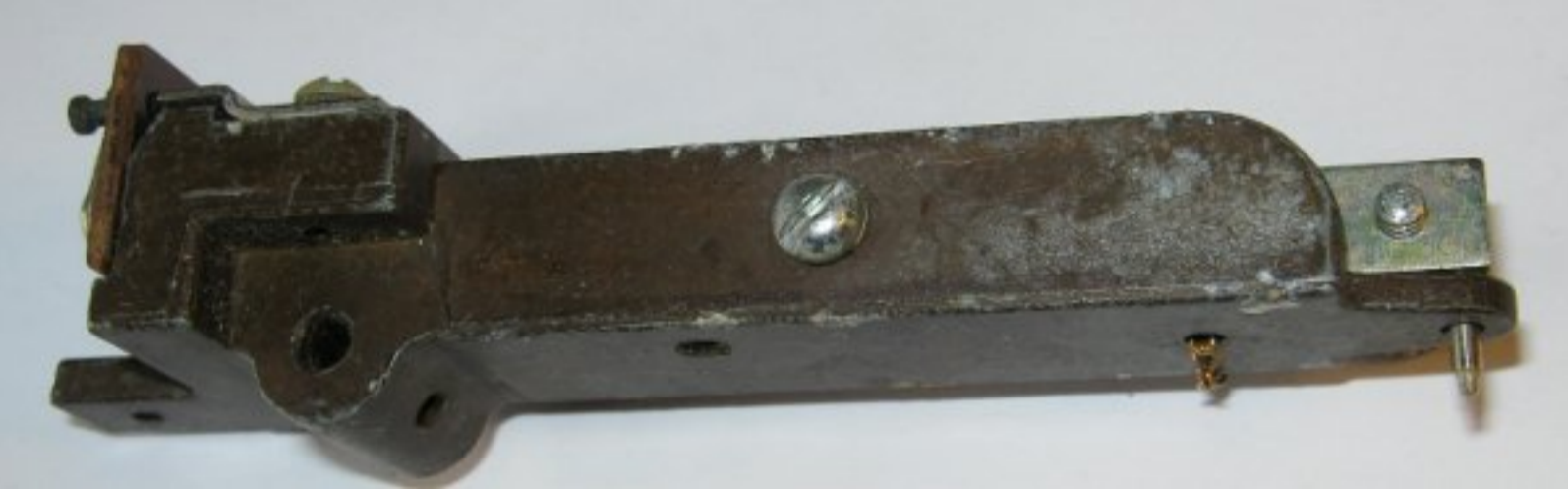
Above and below: view of the valve mounted in a phono pickup
