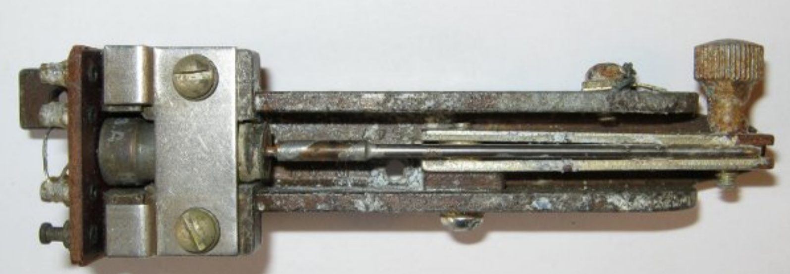
Above and below: view of the valve mounted in a phono pickup
