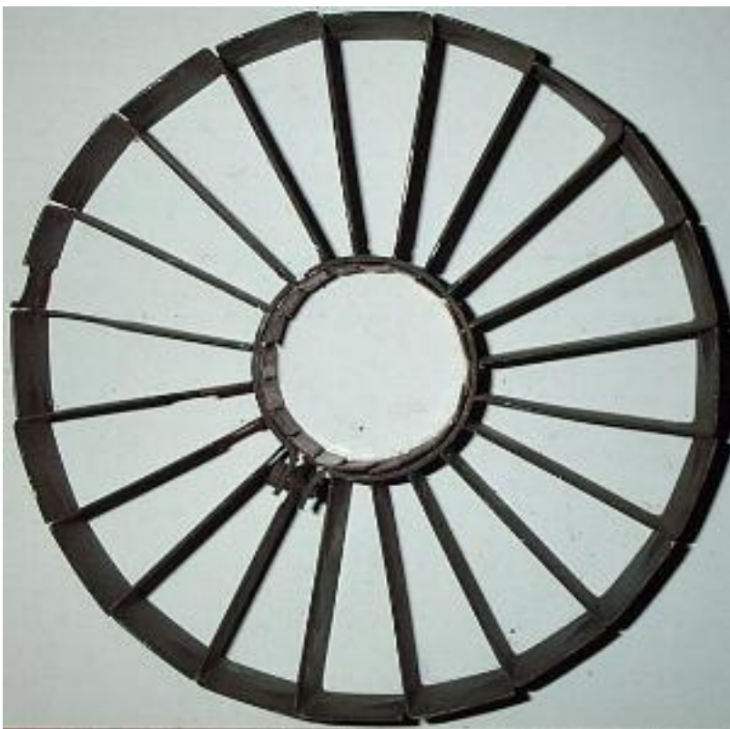
Above: One of four sets of cooling fins assembled. There are 20 fins per ring and 4 rings in total. Below: The fins themselves. The cut-out is to allow access to the screws holding the assemblies onto the anode.
