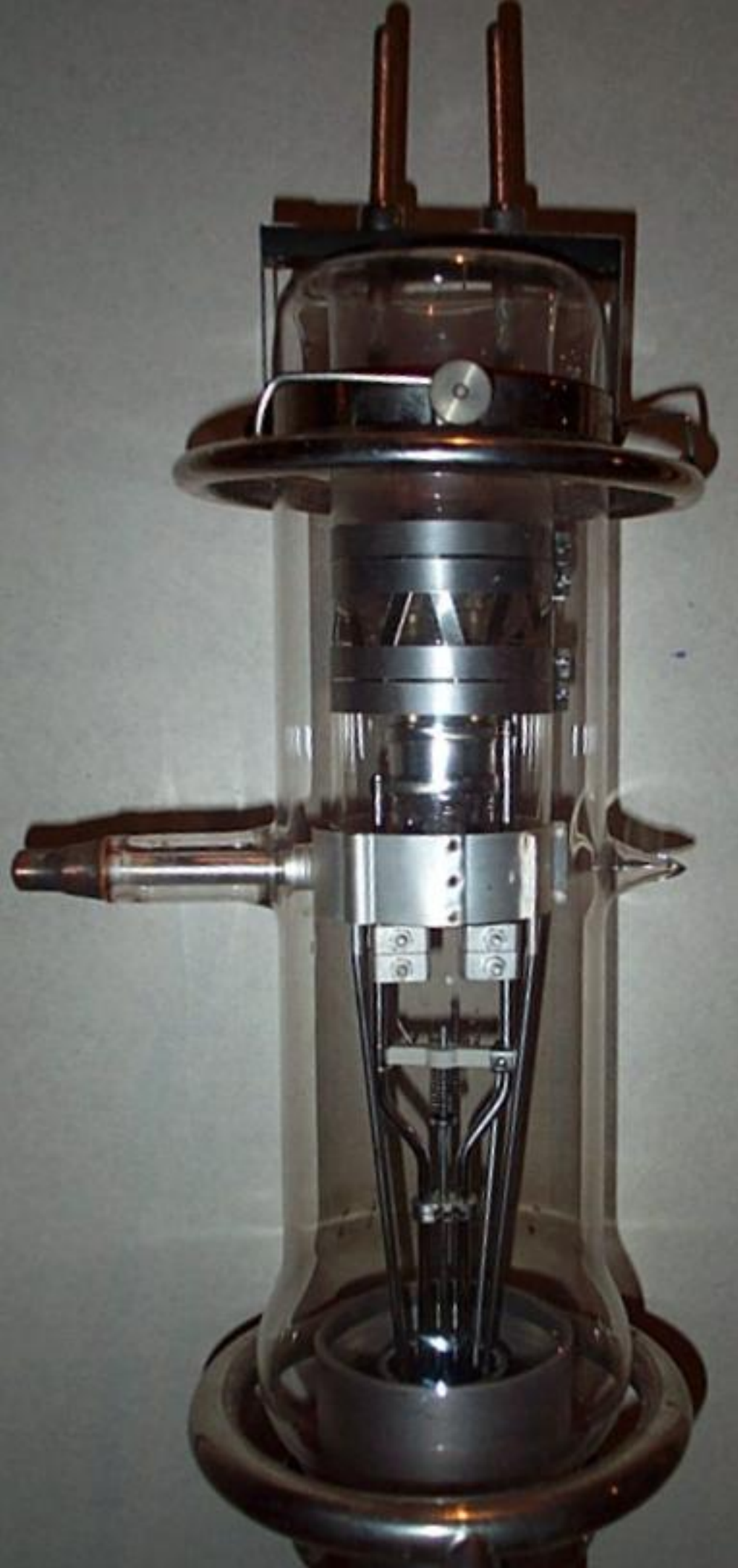
The CAT9 was used extensively by the BBC and others. It was also used in pairs as an intermediate amplifier in the SWB18 100kW shortwave transmitter.
