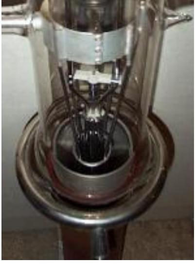
The CAT9 was used extensively by the BBC and others. It was also used in pairs as an intermediate amplifier in the SWB18 100kW shortwave transmitter.
