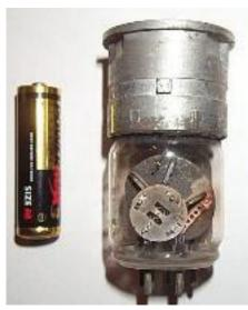
The valve measures 75x39m overall and has a 7-pin base
