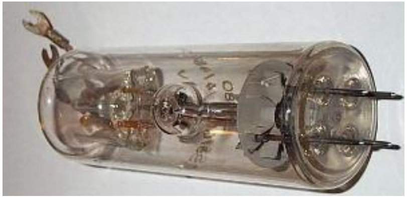
Internal view showing the filament connection. The spiral filament can just be seen above the Telefunken logo.
