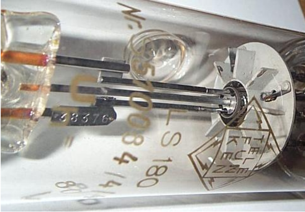
Internal view showing the filament connection. The spiral filament can just be seen above the Telefunken logo.
