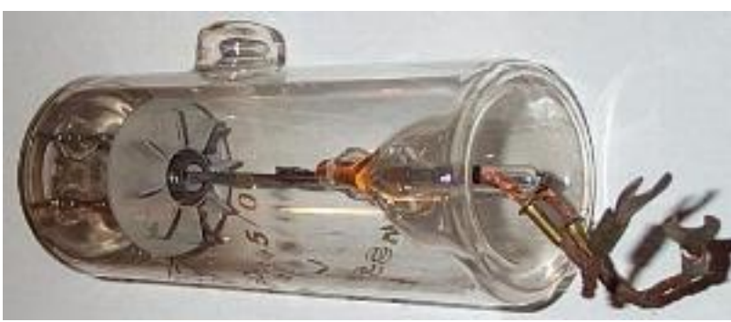
Internal view showing the filament connection. The spiral filament can just be seen above the Telefunken logo.
