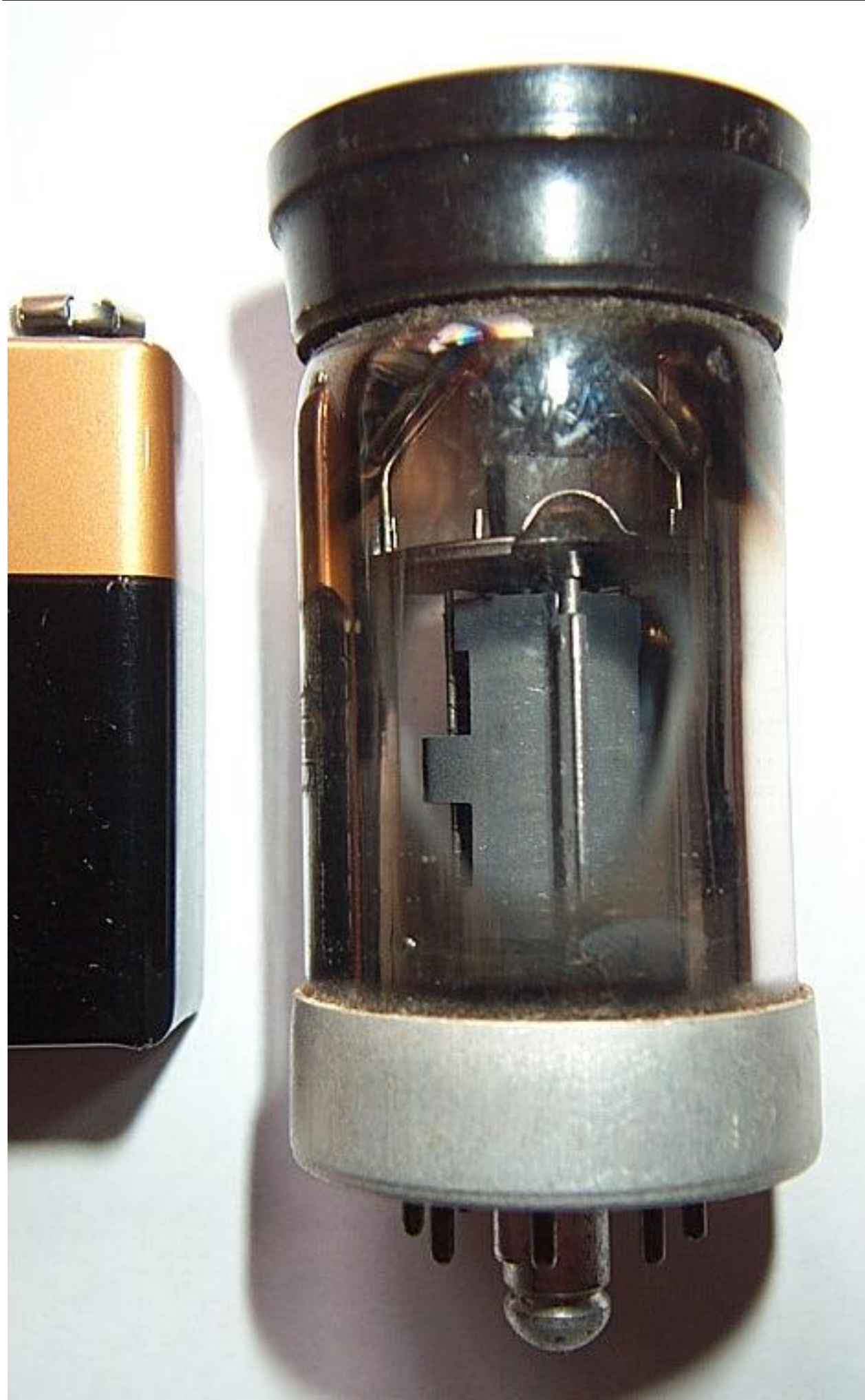
LV1 pentode, 12.6V/210mA heater, 250V anode.
