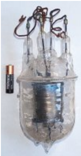
This valve measures 230x100mm overall
