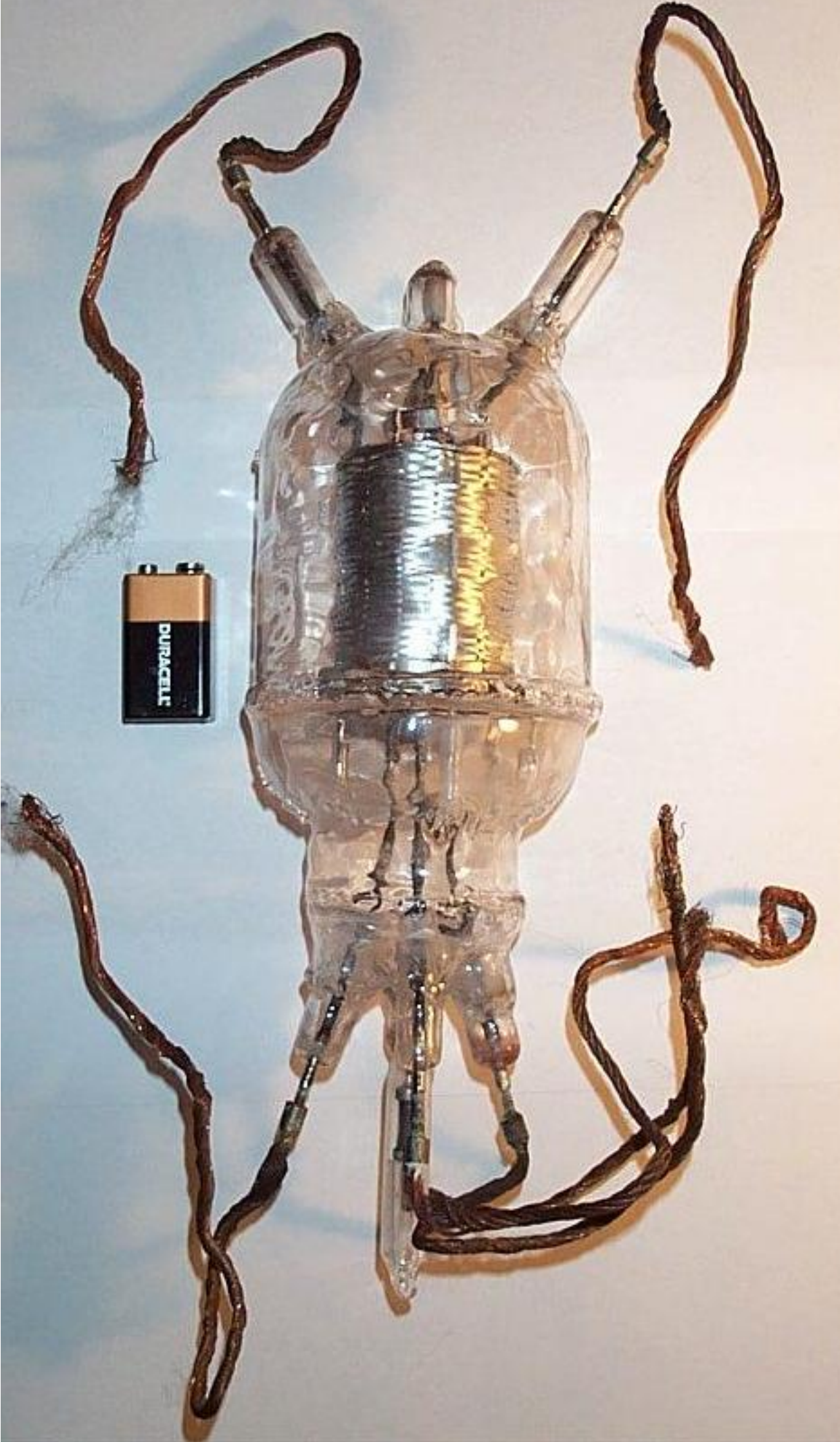
Filament connections and the filament tensioning spring.
