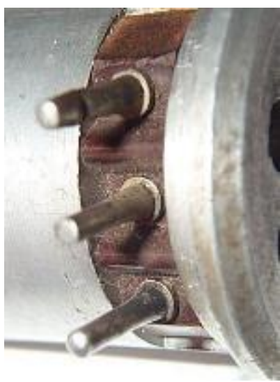
Above: views of the magnetron. Below: detail of the connections and retaining mechanism.
