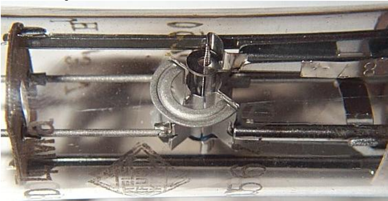
This magnetron is a split anode device, the anode being in 4 segments with opposite segments connected together.
