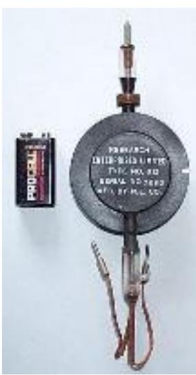
The magnetron measures 190x75mm overall, plus leads, and weighs 550g.
