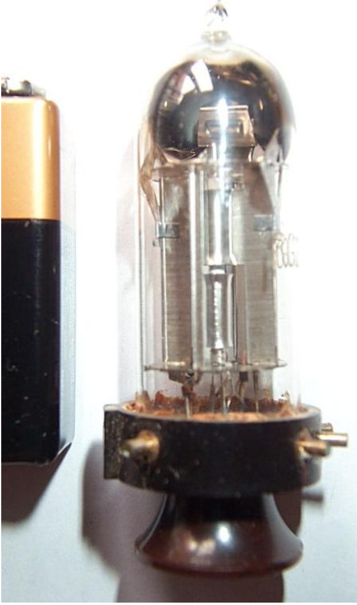
RG12D60 full wave rectifier, 12.6V/200mA heater, 300V/60mA operating.
