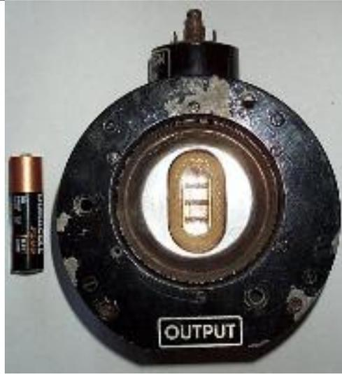
This klystron measures 108x135x47mm overall and has an 8 pin base.
