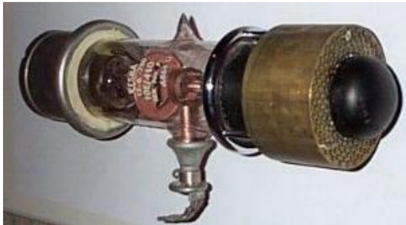
A view of the main glass body of the valve, showing the filament leads from the right and the grid connector at the top of the picture. The grid and a part of the filament can just be seen in the picture on the right.
