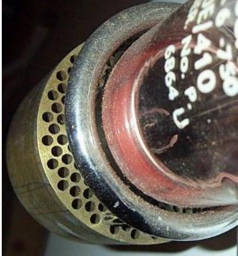
A view of the main glass body of the valve, showing the filament leads from the right and the grid connector at the top of the picture. The grid and a part of the filament can just be seen in the picture on the right.
