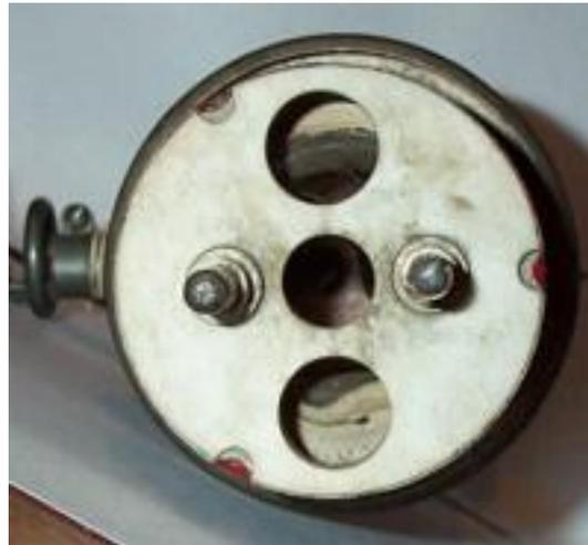
Anode and base view. The figures 2663 are stamped into the centre dome. View into the anode. The grid can be seen.
