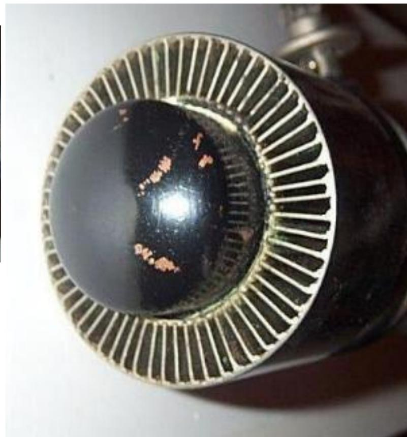
Closeup of a VT98 made by Westinghouse, showing the Air Ministry markings and 'Made in Canada'. The internal structure differs from the VT98s shown above, and the exhaust pip is in the base, rather than on the side of the main glass tube, and this results in a different internal arrangement. The anode cooling is made up of fins, as opposed to the drilled more solid block of the other examples.
