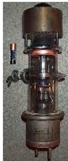
The valve measures 350x85mm overall, plus the grid connection, and weighs just over 2kg. The anode cooling block is 85x50mm. The grid connector extends approx 43mm from the glass, not including the flexible braid.
