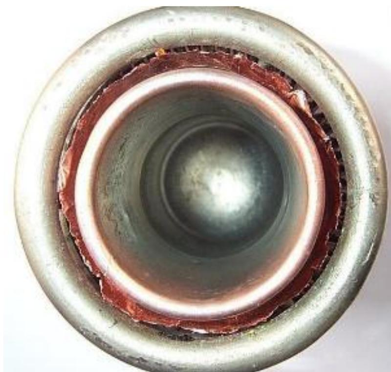
Three pictures of a dissected VT98 valve, this particular one being a Westinghouse made valve. The inside of the anode can be seen, along with the filament and the grid. This is from a Westinghouse made valve.
